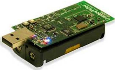
Fig. 12 Crossbow’s TelosB Mote (TPR2420). Our micro-benchmark and trace-driven experiments utilize the energy model of the TelosB sensor device and the CC2420 radio transceiver.
